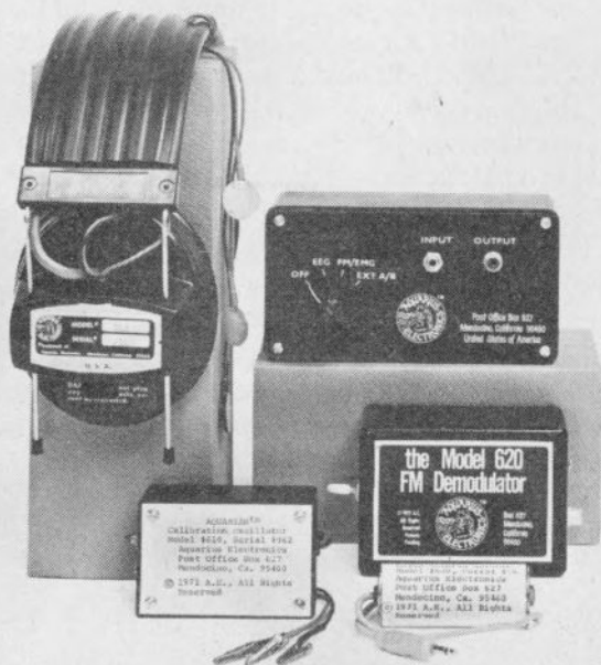
ALPHAPHONE® Headset, 501 Photon Coupler, Calibration Oscillator, FM Demodulator, and Pulse Forming Network.
