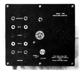
The Model 1508 pentatone adaptor emits a different tone for each brainwave state detected by one brainwave analyzer, plus a tone for artefacts.
