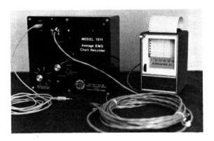
The Model 1511 is a one-channel chart recorder with slow moving paper to record average EMG. It connects to a Model 300B. The Model 1513 records on one channel the amount of time spent in one brainwave category and is used with a brainwave analyzer.
