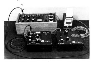
The Model 1512 is a two-channel chart recorder. One channel records the percentage of time spent in one brainwave category. The other channel records the average EMG or muscle tension. It is designed to be connected to a Model 300B EMG and to a brainwave analyzer. It uses slow moving paper.
