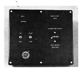
The Model 1509S timer, which uses a mechanical counter, instead of an electronic circuit and seven-segment lighted displays, will display the amount of time in seconds and tenths of seconds spent in each of two categories, similarly to the Model 1509AS. Again, if one timer is not plugged in, it will show simple elapsed time.
