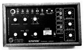
can set frequency ranges for four categories of brainwaves, and the instrument will analyze each brainwave cycle, one at a time, and put it in a category, lighting the appropriate light at that time.
