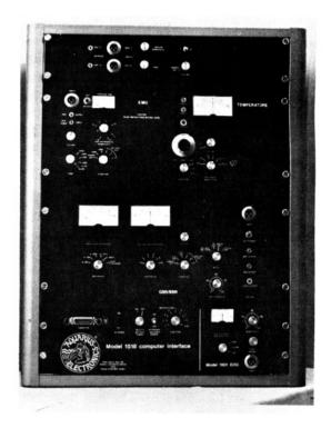
The Model 1518 computer interface is an example of the latter device. It is designed to interface two high speed signals, such as brainwaves, and five low speed signals, such as skin temperature change, average EMG, eye movement, GSR or BSR, to a computer. The high speed signal is sampled and digitized at least 120 times a second. The slow speed signals are sampled and digitized 12 times a second.
